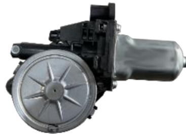
Fig. 1. Second Hand Power Window as Actuator.
