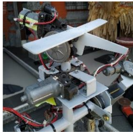
Fig. 7. Two DOF Neck Joint Implementation
